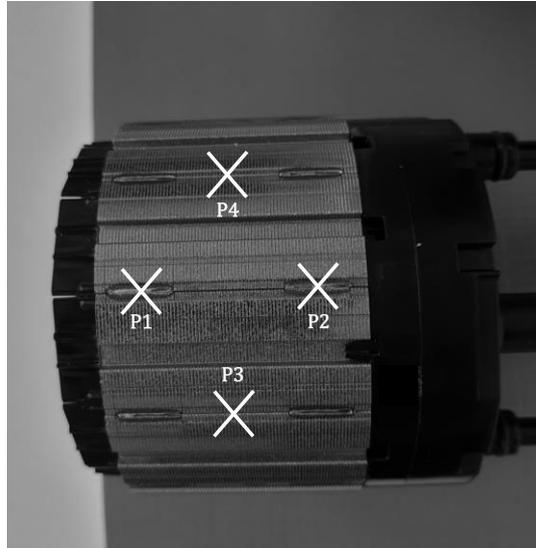
Fig. 4-14 - Grounding point locations in e-ACC stator
